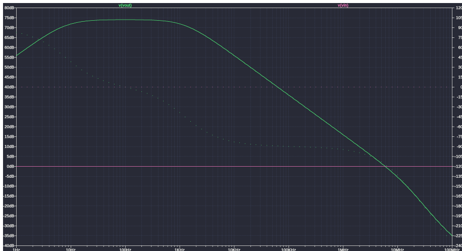
Figure 14: Bode Plot for RC Method of measuring open-loop gain
