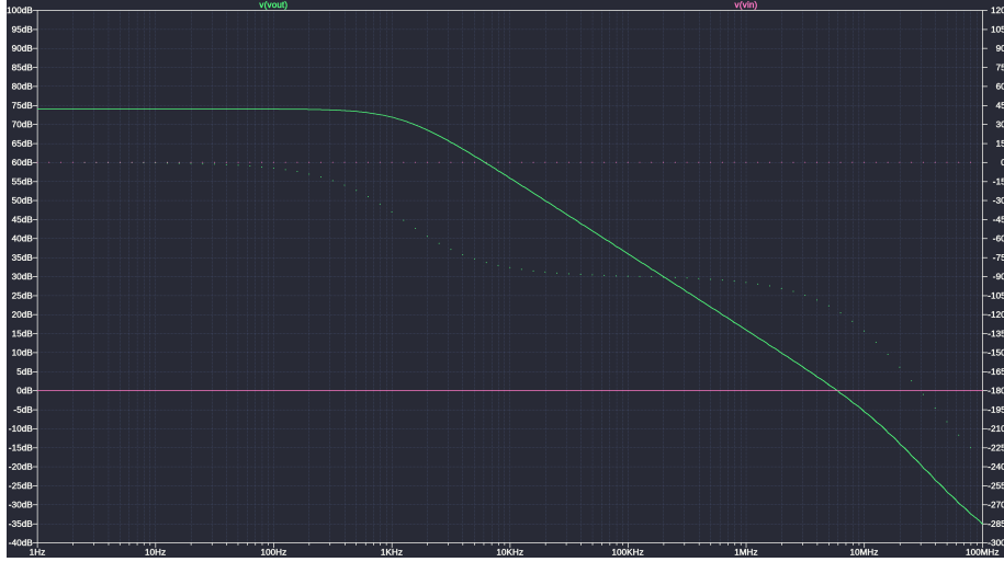
Figure 12: Bode Plot for LC Method of measuring open-loop gain
